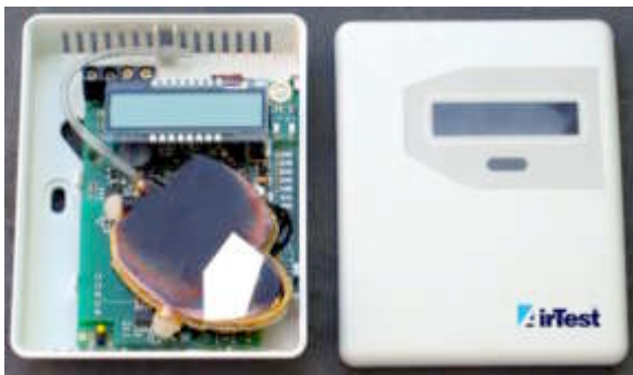
Figure 3: Infrared Dew Point Sensor
